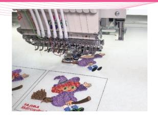
The cutting device can be equipped on TMCR-VF series. As the cord can be automatically cut at the timing of color change, the productivity of multi-colored code embroidery is drastically improved.
