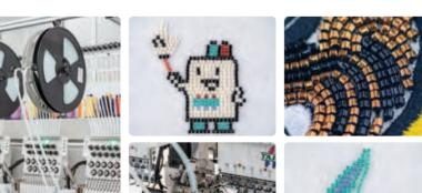
Automatic Color Change Glass Bead embroidery device. It is automated allowing you to embroider beads rapidly instead of by hand so that mass production becomes possible. Also, the beads are set in a tape reel so it is easy to exchange and manage.
